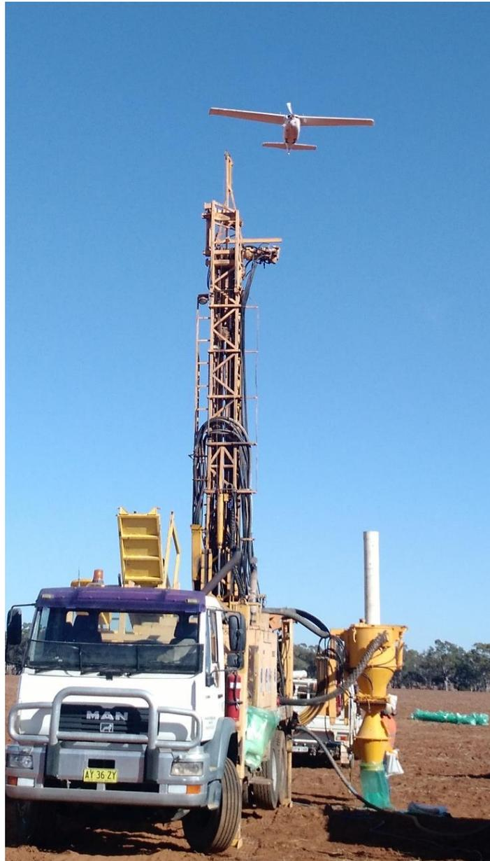
*Figure 1: Maiden drilling program and air-borne magnetic survey at Tiger's Creek Prospect*
